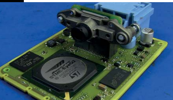
A MobileEye EyeQ2 chip used in a Hyundai Lane Guidance camera module
