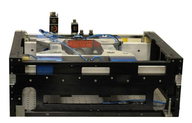
The test rig - a simplified version of a linear motion system
