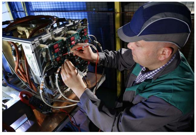
Making measurements in the lab on the new 100kW DC-DC converter
