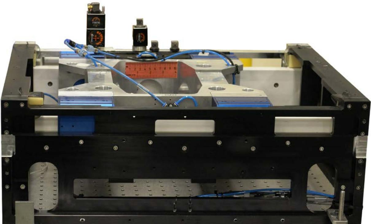
*The test rig - a simplified version of a linear motion system*
