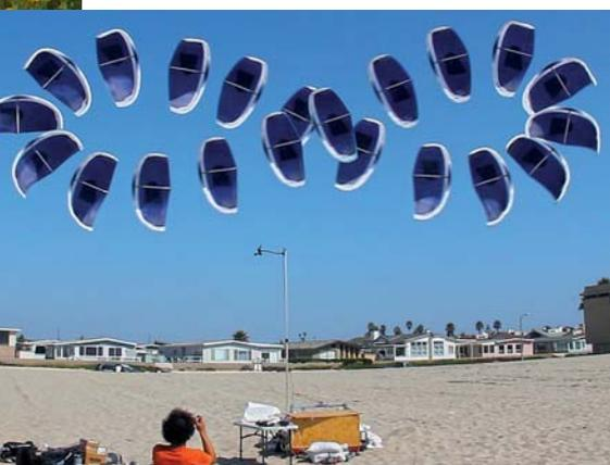
*Small scale prototype built at UCSB with a tethered surf kite flying autonomous cross-wind paths*
