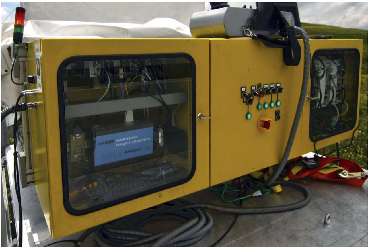
*The controller cabinet during field testing of the FHNW prototype*
