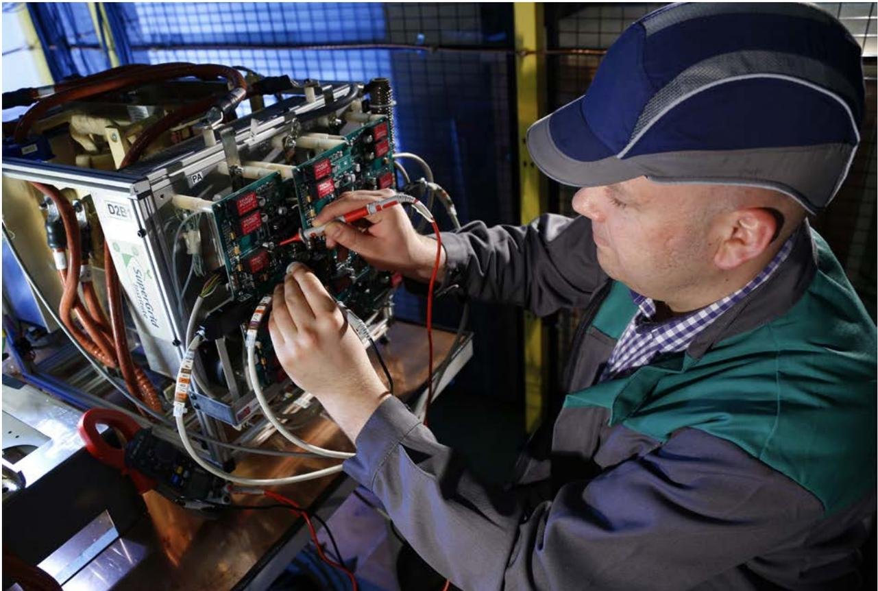
*Making measurements in the lab on the new 100kW DC-DC converter*
